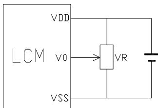
V<sub>DD</sub>-V<sub>0</sub>: LCD Driving voltage
