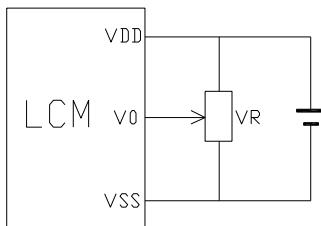
V<sub>DD</sub>-V<sub>0</sub>: LCD Driving voltage
