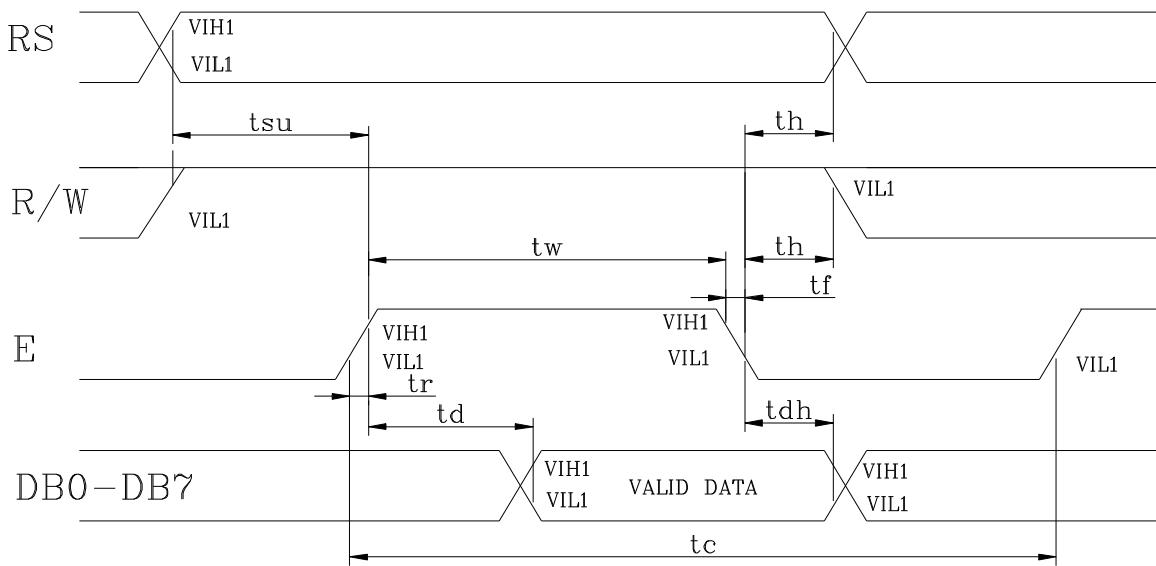
Write cycle ( $T_a=25^\circ\text{C}$ ,  $VDD=5.0\text{V}$ )
